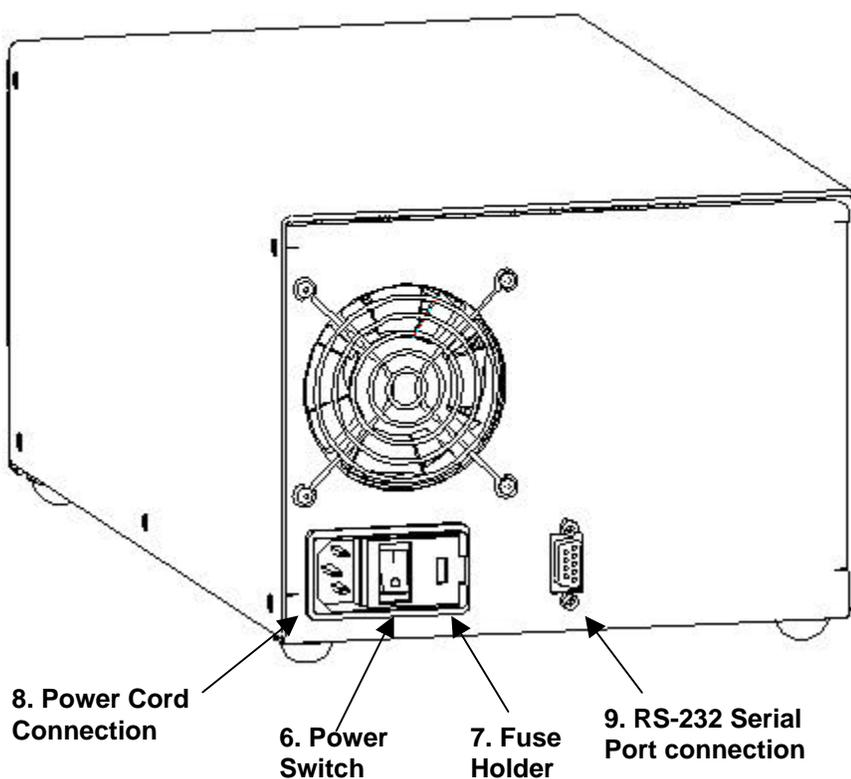
6. **Power Switch.** ON/OFF switch is located on the back panel of the instrument.
